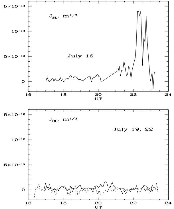
**Fig. 17.** The evolution of the surface layer turbulence on three nights. The integral of  $C_n^2$  from 1.9 to 3.4 m,  $J_{SL}$ , is plotted. On July 16 (top) very strong surface layer turbulence was present in the second half of the night. On the nights of July 19 and 22 with good seeing (bottom, full and dashed lines respectively), little turbulence in the surface layer was detected
