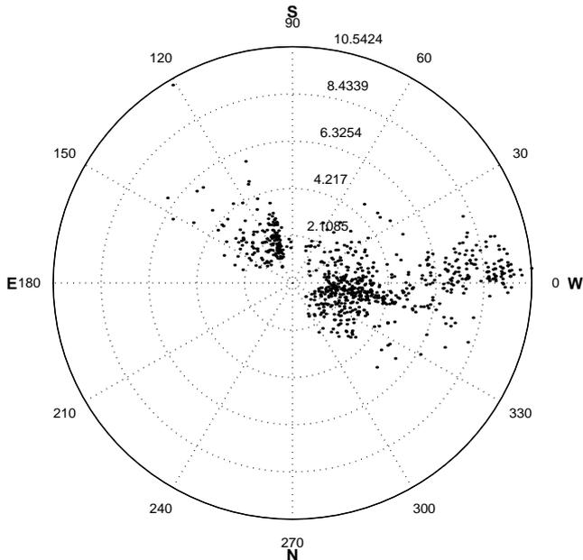
**Fig. 9.** Direction and velocity of the wavefront for the whole GSM mission data set, plotted as a polar diagram. The western wind of low to moderate velocity was predominant, with south-east winds being less frequent
