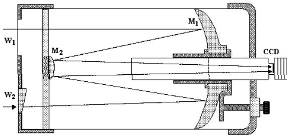
**Fig. 2.** Optical scheme of the Differential Image Motion Monitor (DIMM): M1, M2 are the parabolic primary and hyperbolic secondary mirrors, W1 and W2 are the entrance apertures. Two stellar images are separated on the detector by a wedge prism on W2
