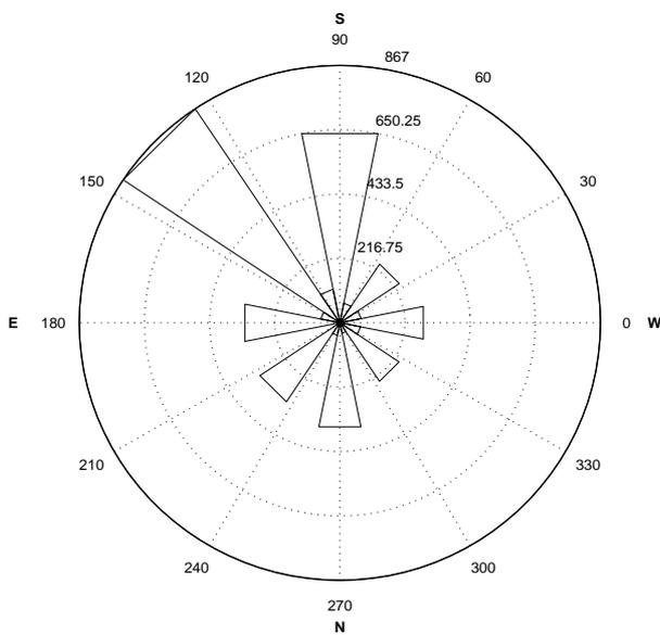
**Fig. 13.** Maidanak windrose measured at 5 m above ground
